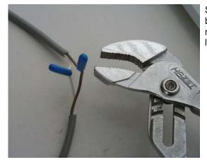
Splices must be done very carefully by means of the enclosed blue silicone sleeves. Tracking current between conductors will result in indication error. Connection terminals will create problems in the course of time and should therefore not be used.
