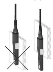
For optimum mounting of the sensor, use mounting clip or mount it free-hanging in the cable
