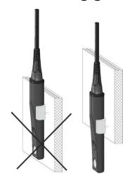
For optimum mounting of the sensor, use mounting clip or mount it free-hanging in the cable.
