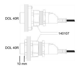
The sensor is mounted so that at least 10 mm of the sensor end is free.
