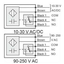
Supply voltage is connected to the blue and brown wire.
